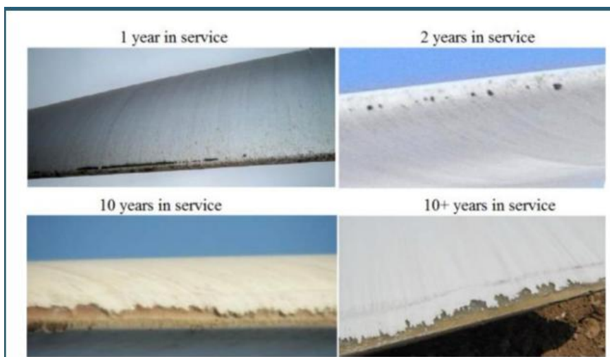
Figure 6. Examples of leading edge erosion in the field across a range of years in service. Source: [25]
